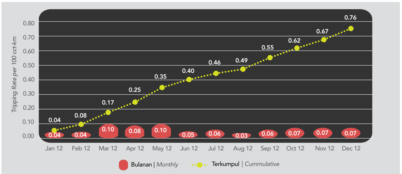
Carta 2: Insiden Pelantikan bagi Talian/Kabel per 100 cct-km Bulanan Carta 2: Monthly Tripping Incidents for Lines/Cables per 100 cct-km
