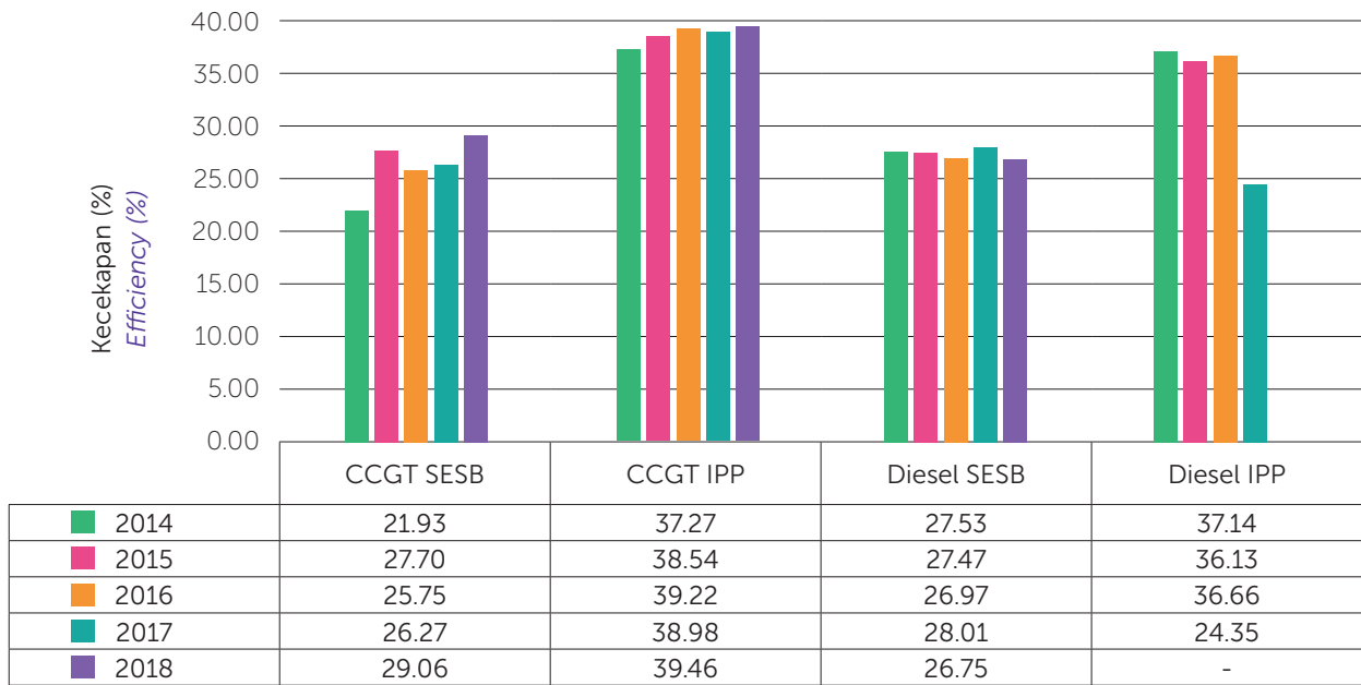
Purata Kecekapan Thermal Mengikut Jenis Loji Jana Kuasa di Sabah Average Thermal Efficiency by Type of Power Plants in Sabah
